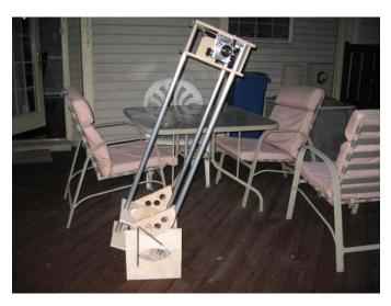
Last month we profiled a Crayford focuser built by Prasad Agrahar, a student at the NCA Amateur Telescope Making class. Here is Prasad's focuser again, during first light on his assembled 8 inch Dobsonianmounted Newtonian reflecting telescope.
